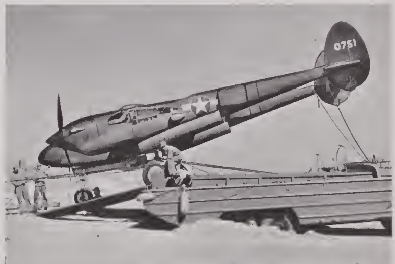
FIGURE 77. P-38 rolling down ramp to beach after DUKW ferry trip.
